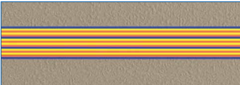
LAYERS OF FUNCTIONAL MATERIALS ARE MULTIPLIED. Shown here is microlayer structure before outer or skin layers are added. Brown areas at top and bottom represent metal of flow channels. Blue, yellow, and orange microlayers represent, respectively, material with active component such as oxygen scavenger; adhesive; and barrier polymer.
