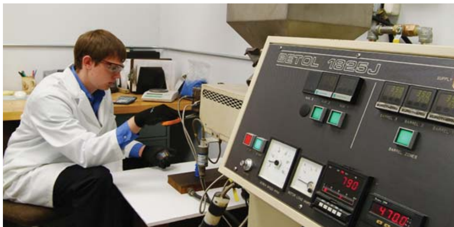
KEY TO OPTIMUM DIE PERFORMANCE is rheology, the study of flow. In EDI's rheology lab, shown here, sophisticated instruments are employed to determine how specific polymers flow under certain defined forces encountered inside a die. EDI engineers use this knowledge to design a die that provides optimum flow under the processing conditions anticipated by the customer.
