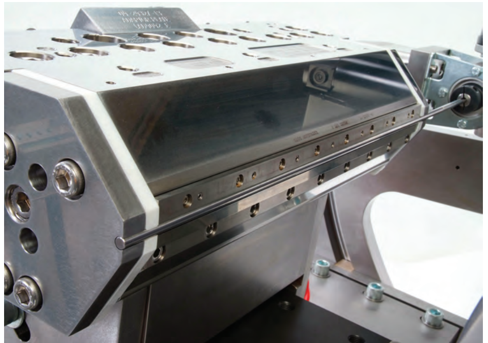
NEW DIE RUNS PSAs 'THIN AND FAST.' Easily visible in the lip area of this die is a motorized rotary rod that allows gels to pass through the lip opening and the coating interface, preventing buildups that cause streaking. Another new feature, inside the die between the manifold and the lip opening, is a restrictor bar for adjusting the coat weight profile. The die makes possible coat weights as low as 0.5 mil (0.0127 mm) and line speeds up to 2,000 feet/min. (610 meters/min.).
