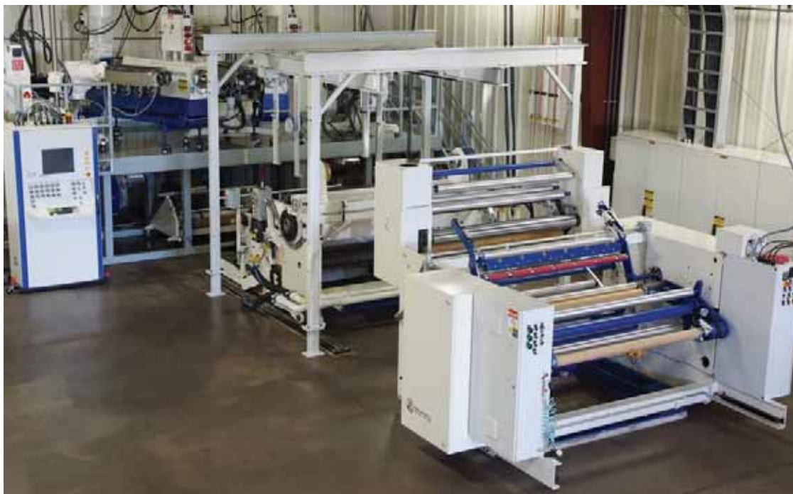
LARGE PROCESSING LINE FOR FILM, COATING, AND LAMINATION. This new multi-process line at EDI's Technology Center has five extruders and can produce single- or multilayer film up to 1.6 meters wide at thicknesses from 8 to 125 microns. Speeds at 8 micron thickness range up to 750 feet (230 m) per minute. The line can also be used for extrusion coating or lamination. Two unwind stations permit converting of film made on the line or shipped to EDI as rollstock. Besides using this and other processing lines at the Center for its own research, EDI rents them to companies looking to do trial runs without tying up their own equipment.
