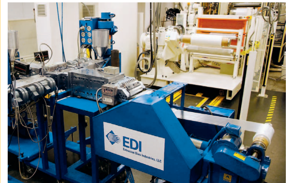
LABS THAT SAVE MATERIAL AND PREVENT DOWNTIME. Laboratory extrusion line shown here is one of three at EDI’s Wisconsin headquarters that customers can rent for product development and testing. Lines are for film, extrusion coating, and slot die coating.
