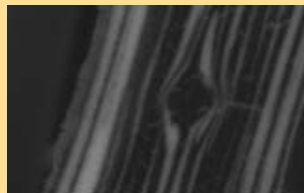
FEWER WEB BREAKS occur with microlayer film because gels and other defects are more likely to be encapsulated, as shown here.
